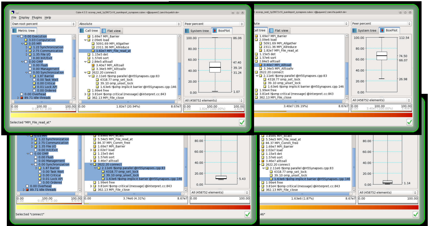
Figure 5: Scalasca analysis report explorer views of import_synapses extract of a Score-P measurement profile from NEST-import execution on all 28 racks of JUQUEEN (28 672 MPI ranks each with 16 OpenMP threads). The upper-left view shows 21% of time is in MPI_File_read_at , when loading 1.9 TiB of HDF5 neuron and synapse data in six parts (174 calls). Reading time by rank varies from 1.07 to 86.06 seconds, resulting in up to 85 seconds of waiting within the subsequent synchronising collective MPI_Alltoall (upper-right), as part of the 120 seconds each rank takes to load and redistribute the data. The lower views show time in the subsequent connect step ranging from 4.14 to 52.62 seconds, where some threads wait up to 48 seconds in the implicit barrier closing the OpenMP parallel region.
