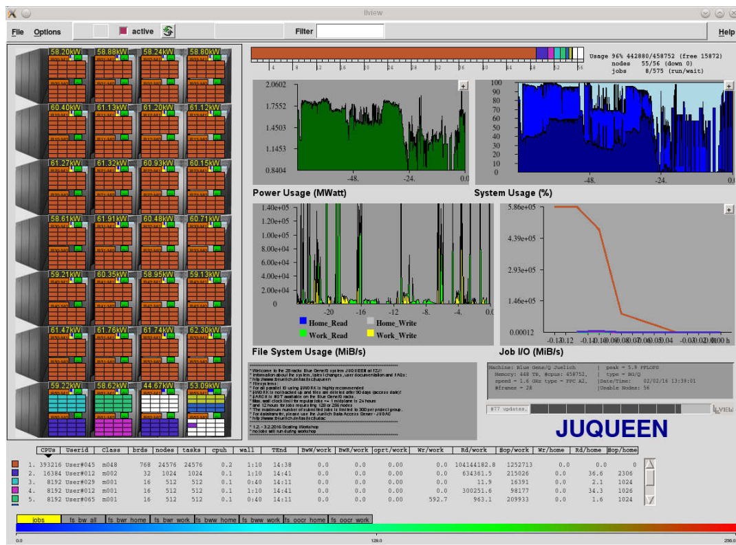
Figure 7: LLview monitoring of JUQUEEN during workshop during an execution of CIAO on 24 racks (and several smaller jobs), with charts of the CIAO job file I/O bandwidth (middle right), file-system usage of the previous 24 hours (centre), and three-day histories of power usage and job-size mix (centre and upper right).
